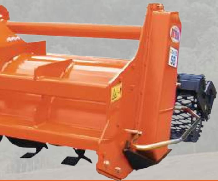
Recommended especially to work and improve stony soils in agriculture, greenhouses, parks, gardens and golf courses. A special screening system safely separates and deposits the stones picked up from the soil underneath the seed bed. Fine soil remains on top. Light and medium models are available for working in parks, gardens and the heavier model designed to work in particularly heavy conditions and bigger grounds.
